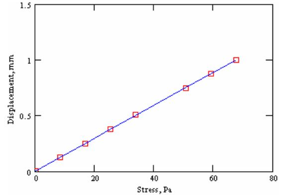
**Figure 8.** Calibration curve for S<sup>3</sup>F composition with shear stress module  $\mu = 117$  Pa.
