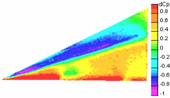
Figure 15. PSP results plotted in  $\Delta C_p$ ,  $V = 20 \text{ m s}^{-1}$ ,  $\alpha = 10^\circ$ .
