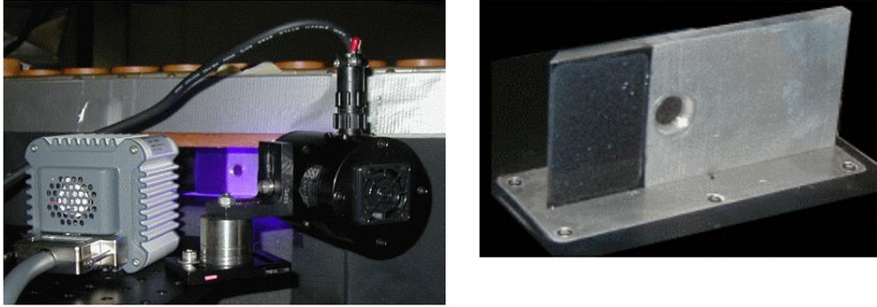
Figure 10. Typical S<sup>3</sup>F experimental set-up (left). Tested model (right). S<sup>3</sup>F cavity has depth of 1 mm (front black part).
