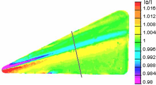
Figure 16. S<sup>3</sup>F results: normal component of deformation field ( $I_o/I$ ); flow velocity  $20 \text{ m s}^{-1}$ , angle of attack  $\alpha = 10^\circ$ .
