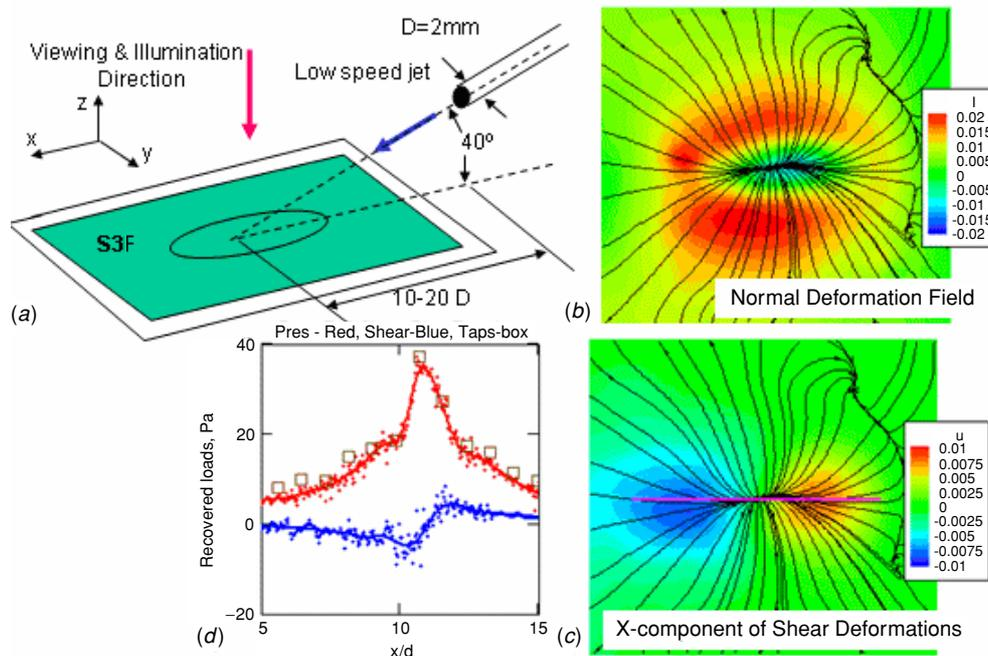
Figure 18. Impinging jet measurements of pressure and shear-force distributions using S<sup>3</sup>F. (a) experimental set-up, (b) normal deformation field, (c) x-component of shear deformation and (d) S<sup>3</sup>F derived shear (blue), pressure (red) and pressure taps (squares).
