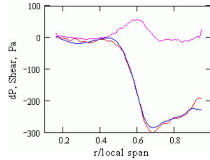
Figure 17. Comparison of S<sup>3</sup>F (blue) data with PSP (red). Pressure variation in section presented in figure 16. Shear force represented by magenta curve.
