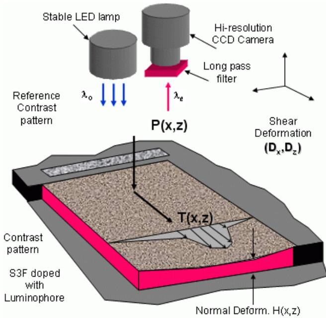
**Figure 7.** General layout of S<sup>3</sup>F image acquisition system.
