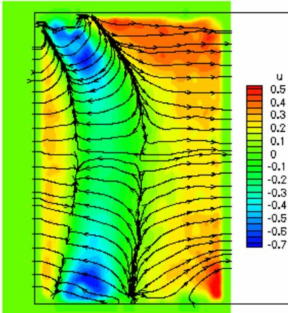
Figure 12. X-component of shear deformation field. Units are in pixels.
