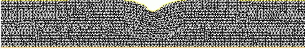
**Figure 3.** FEA solution of load on elastic polymer. Zoomed view of the deformed FEA grid.
