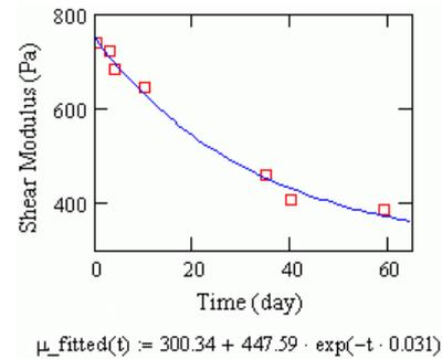
**Figure 9.** Decrease in shear modulus of S<sup>3</sup>F film as a function of time. Film was 1 mm thick with an initial modulus of 735 Pa.
