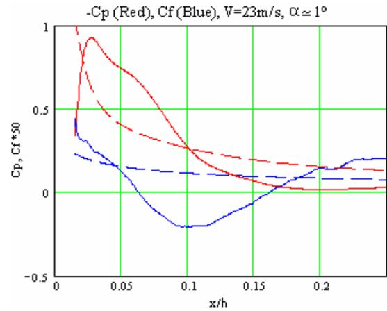
Figure 13. Reconstructed  $-C_p$  (red) and  $C_f \cdot 50$  (blue) distributions compared with CFD (2D potential flow) and Blasius estimations (dashed Lines).  $V = 23 \text{ m s}^{-1}$ , angle of attack  $\alpha \cong 1^\circ$ .
