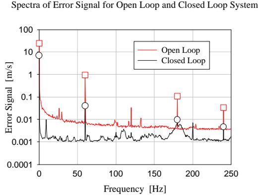
Figure B3 Spectra of the error signal for the open and closed loop systems.
