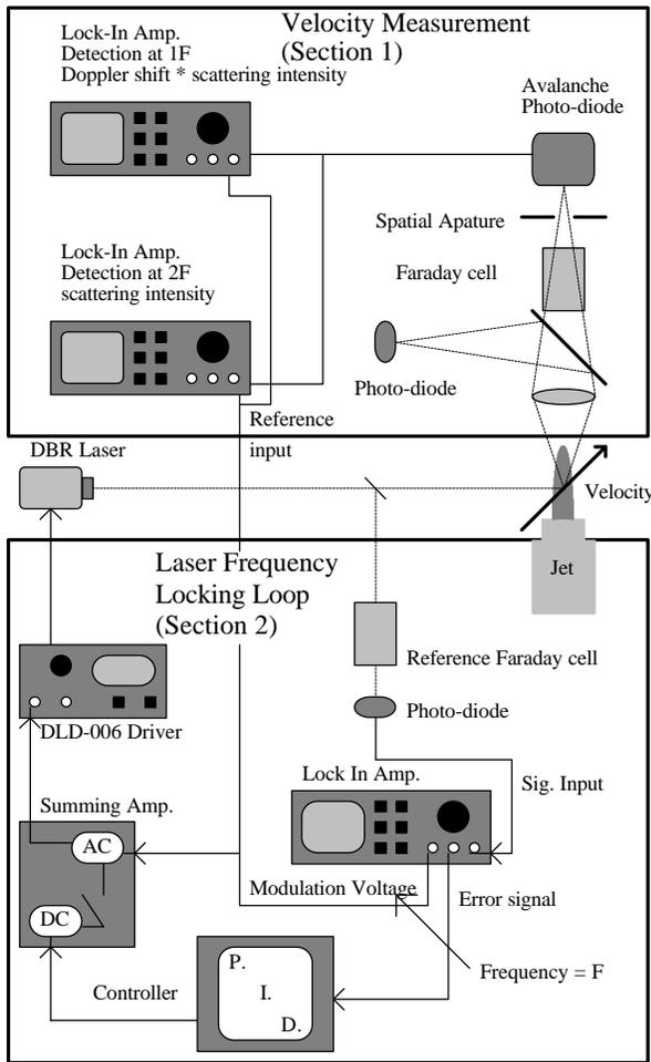
Figure 1 Point Doppler Velocimetry System.
