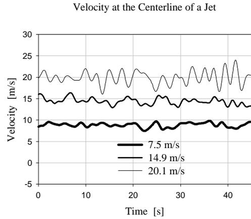
Figure 7 Velocity traces of the jet centerline velocity using the PDV system.
