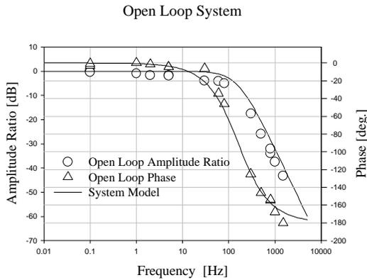
Figure B2 Bode plot of the open loop system compared to the simple model.
