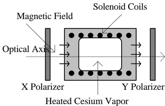
Figure 2 Components of a Faraday Cell.
