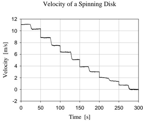
Figure 5 Velocity measurements of a rotating disk using the PDV system. System integration time set to 1 [s].
