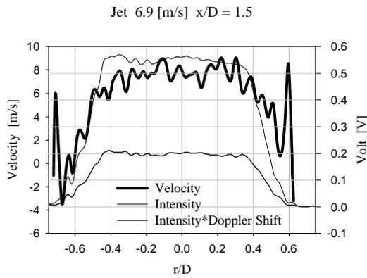
Figure 6 Velocity profile of a jet using the PDV system. System integration time set to 1 [s].
