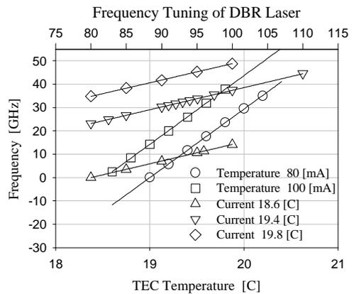
Figure 4 Frequency tuning of the DBR laser using TEC temperature (bottom axis) and operating current (top axis).
