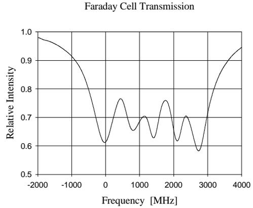
Figure 3 Relative intensity versus frequency for a Faraday cell
