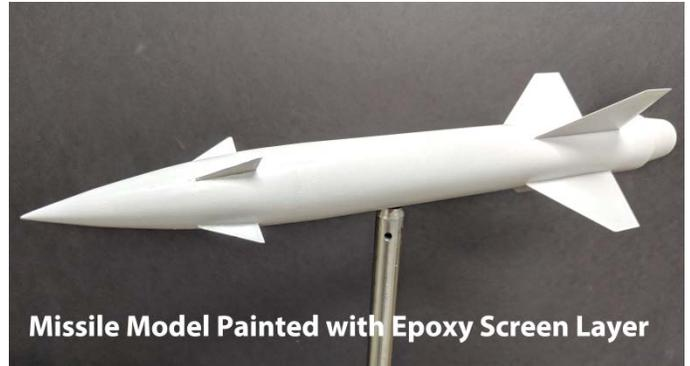
Missile Model Painted with Epoxy Screen Layer
