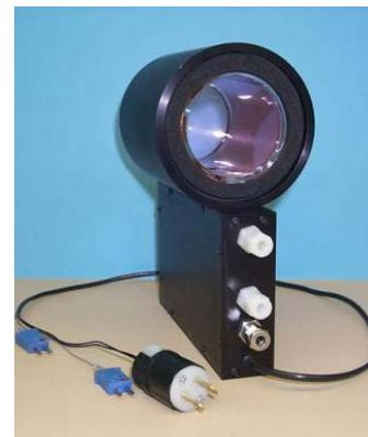
Packaged I2M-10 with thermocouples and heater
