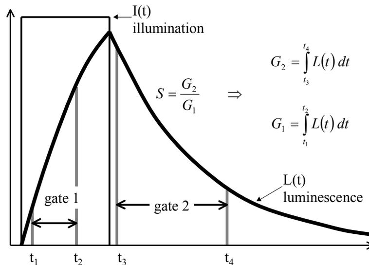
Fig. 3 - Luminescent lifetime of a pressure-sensitive probe, demonstrating the two-gate lifetime measurement approach.
