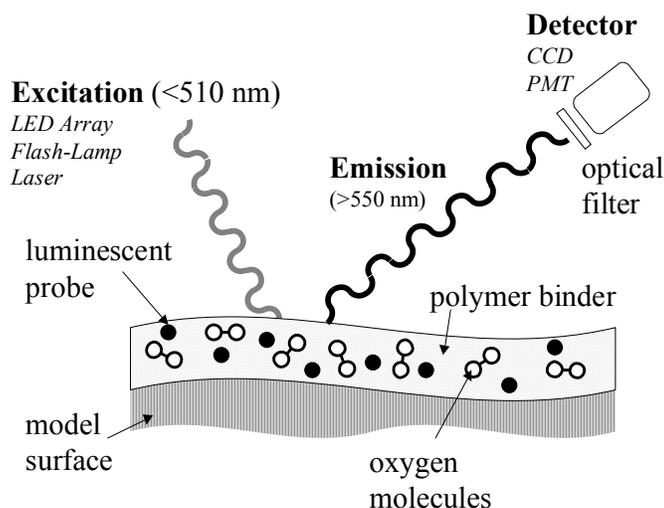
Fig. 1 - Components of a PSP system.
