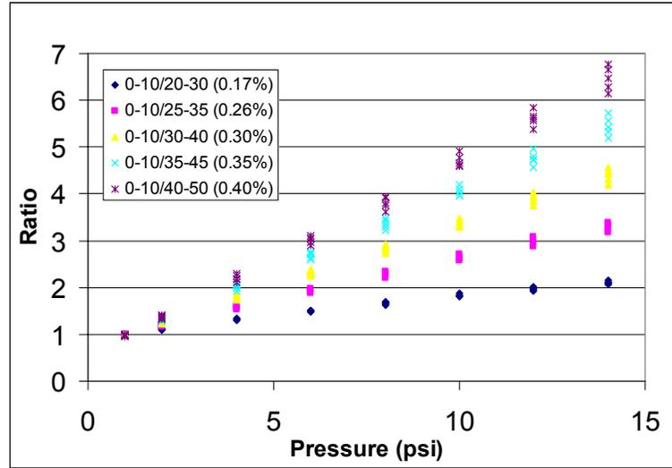
Fig. 4 - Various gate ratios for Pt:TFPP/FIB paint. All gates are in microseconds. Percentage-per-degree temperature sensitivity is given in parentheses.
