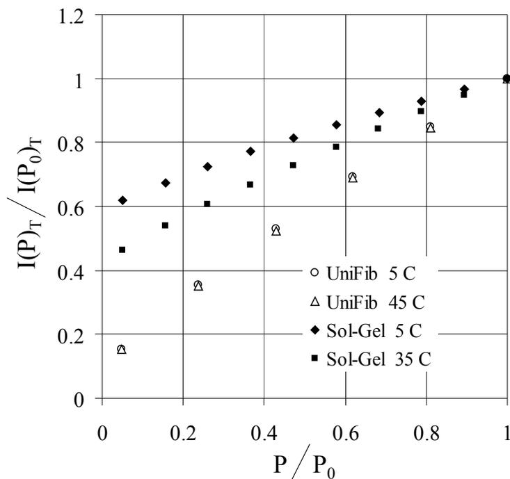
Fig. 5 - Ideality of Pt:TFPP in FIB and Ruthenium-complex in Sol-Gel. Calibration data along each isotherm were normalized using the intensity at that temperature and the reference pressure. The resulting plot shows the sensitivity of the paint at different temperatures.
