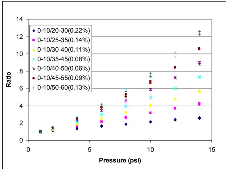
Fig. 7 - Various gate ratios for Pt:FIB/Tc binary paint. All gates are in microseconds. Percentage-per-degree temperature sensitivity is in parentheses.
