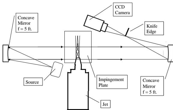
Figure 8 Single pass schlieren system.
