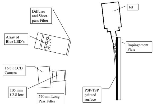
Figure 5 CCD camera based Temperature and Pressure sensitive paint data acquisition system.
