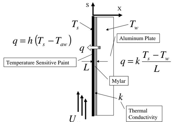
Figure 6 Experimental set up for heat transfer measurement.
