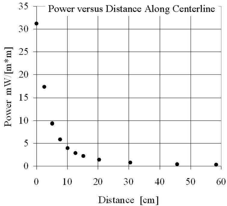
Figure 3: Spectral Irradiance as a function of distance along centerline of an LM2X-400
