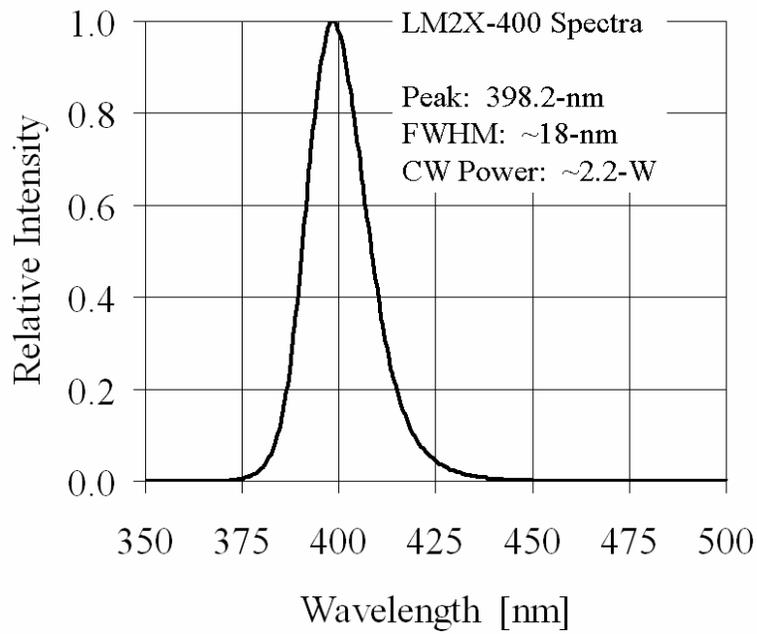
Figure 1: Spectral content of a LM2X-400.
