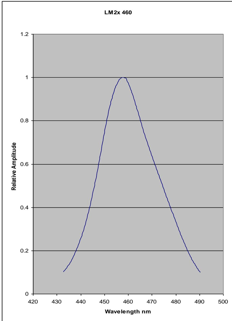
Typical waveform of an LM2X 460
