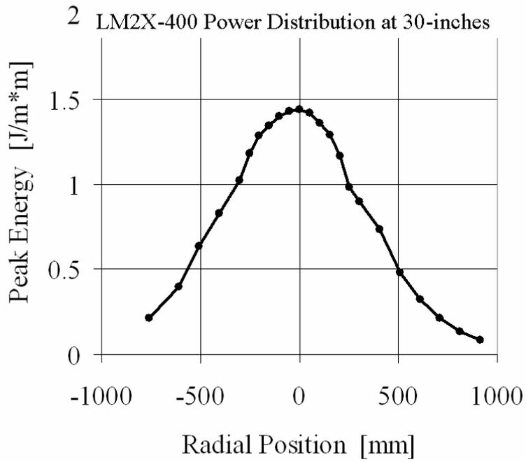
Figure 2: Distribution of radiation at 76-cm (30-inches) for an LM2X-400.
