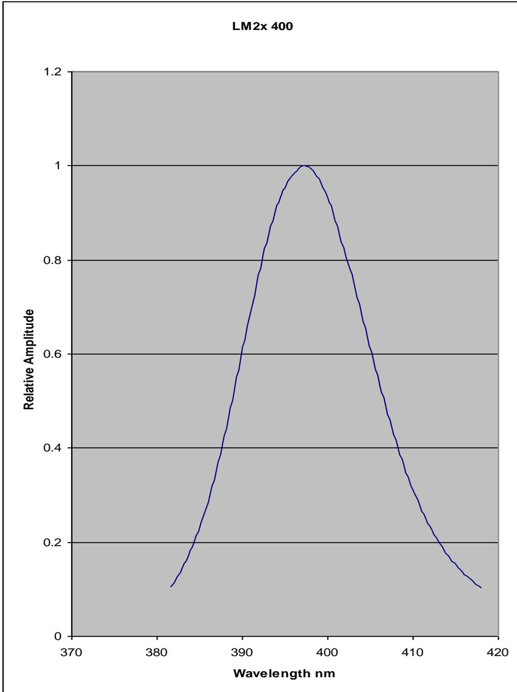
Typical waveform of an LM2X 400
