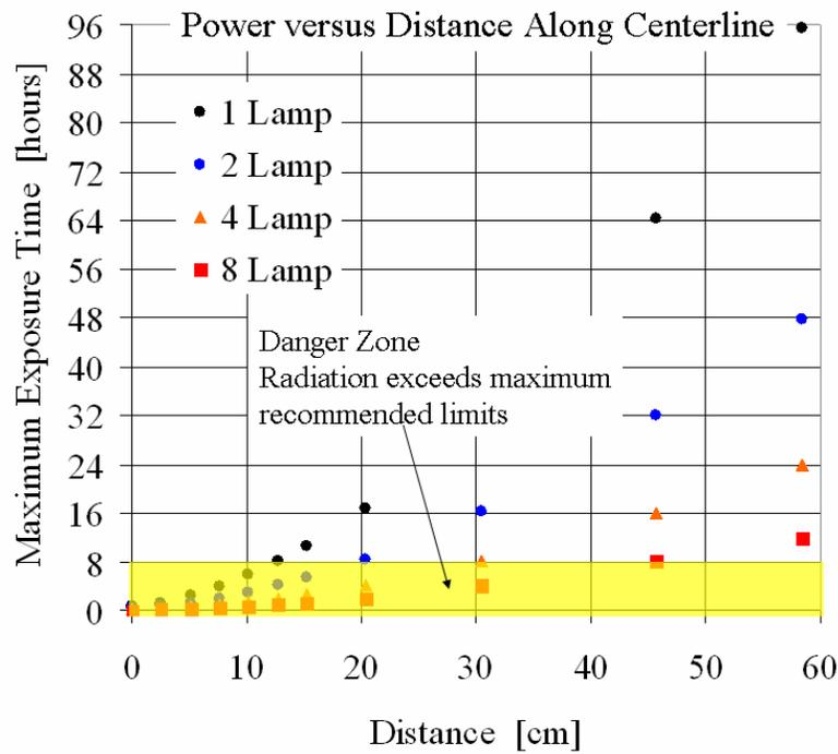
Figure 4: Maximum recommended exposure time limit as a function of distance for an LM2X-400. Note that use of multiple lamps increases the safe working distance.
