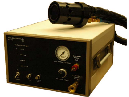
LM2XX-DMHP components: LED head, umbilical, and control box.
